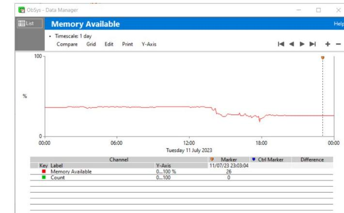
On the comparison view, the lower part of the window shows which colours represent which logs. It also shows the values of the logs at two different points in time – the Marker and the Ctrl Marker
