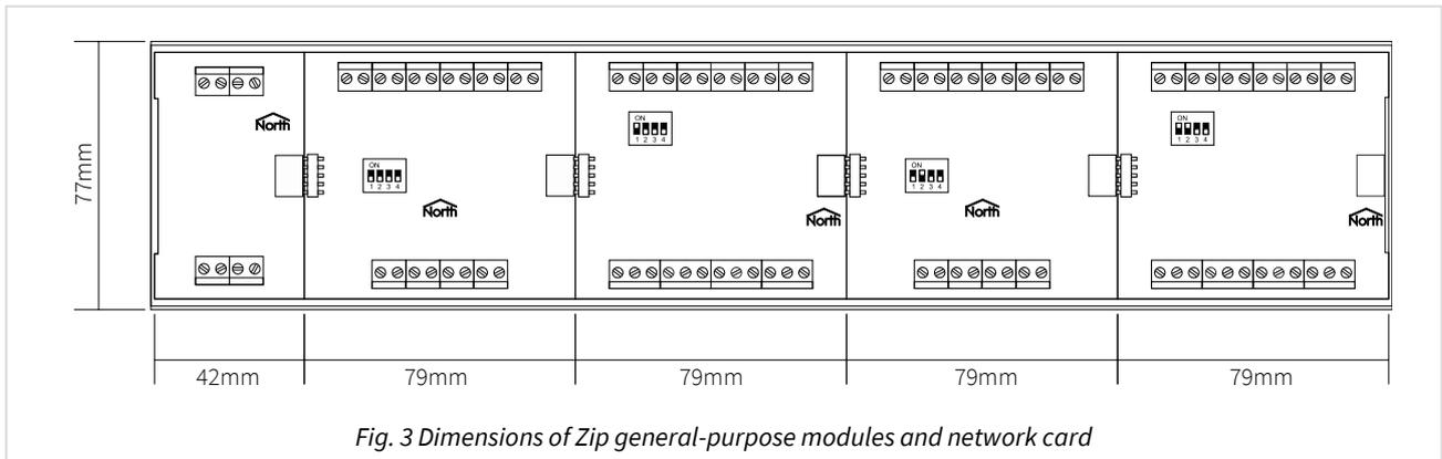
The total width for a network card and a maximum of four Zip modules will be:
