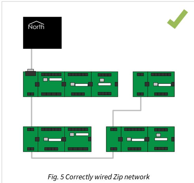
Fig. 5 Correctly wired Zip network
