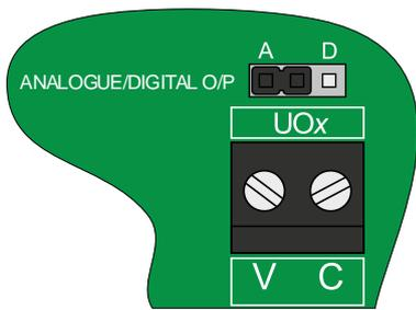
Universal Outputs are used as an analogue output in the range 0-10V, or as a switched 12VDC supply.
