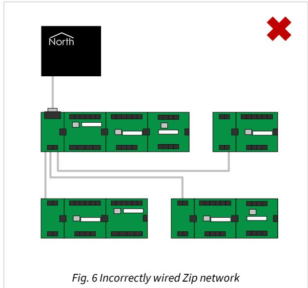
Fig. 6 Incorrectly wired Zip network
