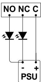
As the relay provides both Normally-Open and Normally-Closed contacts, it is possible to supply voltage to the Common connector and use both Normally-Open and Normally-Closed contacts to energise different circuits. For example, the relay could switch power to either a red LED circuit or a green LED circuit.
