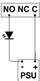
The Common and the Normally-Open connector operate as an isolated switch to provide a switching function in an external circuit. The external circuit could, for example: provide voltage, via the relay, to an LED indicator; provide voltage to a change a contactor (a more powerful relay); or even provide voltage to power a heater.
