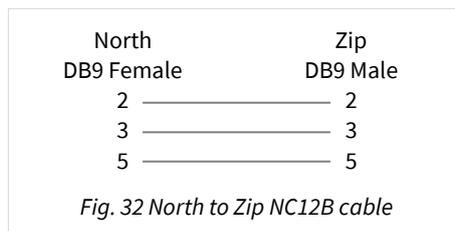
The maximum RS232 cable length is 15m and should be as short possible.
