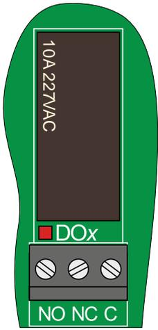
Relay outputs are available on the following modules: *M7002A*, *M7006A*, and *M7007A*.
