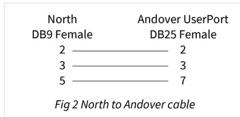
The maximum RS232 cable length is 15m and should be as short as possible.
