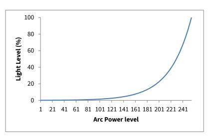
Control devices (such as a North device) may send a command to instruct control gear to change this brightness level, using broadcast, group, or individual addressing. The current level can be determined using individual addressing only. The driver supports both arc power and percent levels.
