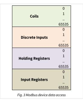
Implementations of the Modbus protocol in a device can vary:
