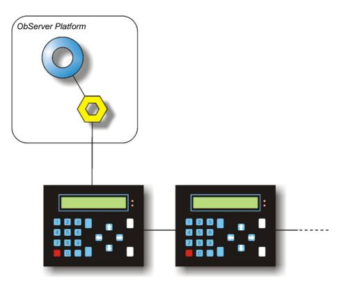
For communications with the NC25-4 to begin, algorithm chip sets of v44.07 or higher should be fitted; these are located on the main board U29 and U30. The GRAPHICS (GRAP) command must also be present in the database chip U28.
