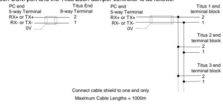
The cable between COM port and the Titus Zeon damper controller is as follows:
