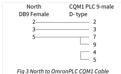
Note: The Omron PLC RS232 9-way connector is non-standard.
