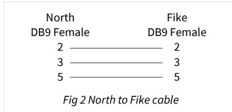
The maximum RS232 cable length is 15m and should be as short as possible.
