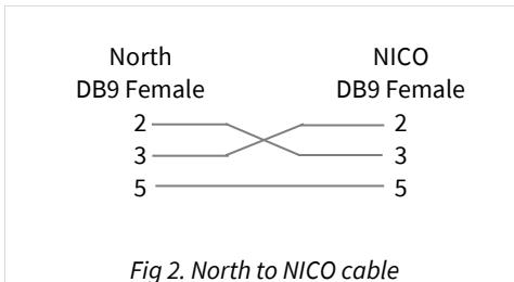
The maximum RS232 cable length is 15m and should be as short as possible.
