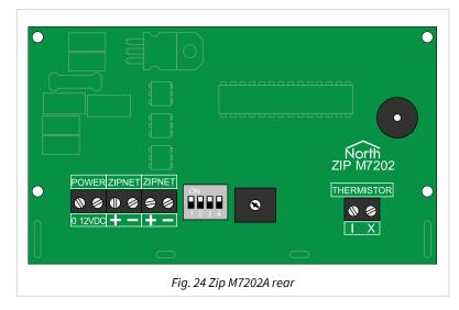
The display fits into a 2-gang pattress or socket box to simplify installation.
