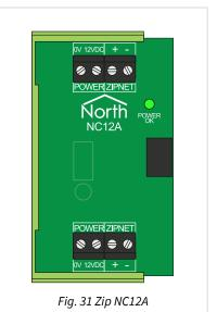
Use either connection to route the power in, and then optionally out via the second connection to another network card. Ensuring the power supply is enough for all modules.
