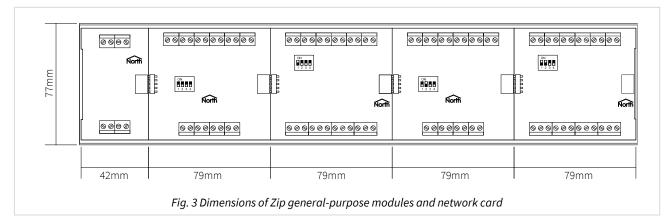
The total width for a network card and a maximum of four Zip modules will be: 42mm + (4 x 79mm) + (2 x 2mm) = 362mm
