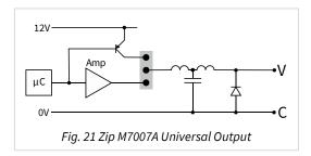
Connect the universal output to 0-10V DC motorised valve, 0-
