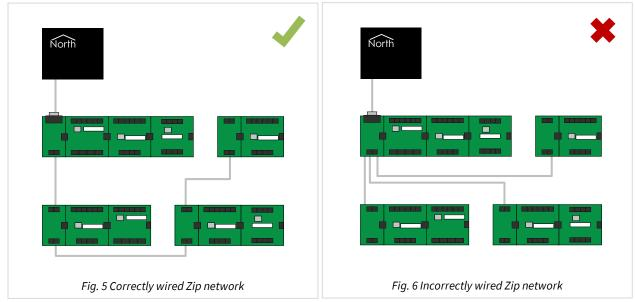
Recommended cables for wiring the Zip network are Belden 8761, Alpha Wire 2401C, or similar shielded twisted-pair cable (minimum 22AWG).
