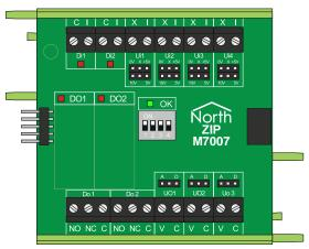
The M7007 is a general-purpose Zip module with a mix of different input-output capabilities, including universal inputs and universal outputs.
