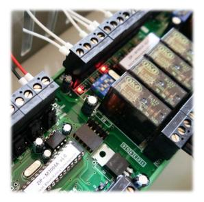
Different Zip modules are available. Some provide general-purpose inputs for measuring, such as volt-free contacts, thermistors, and 0-10 volt analogues. Some provide general-purpose outputs, including relays, switched 12-volt digitals, and 0-10 volt analogues. These modules clip together to fit on DIN rail, thereby simplifying control panel layout and construction.
